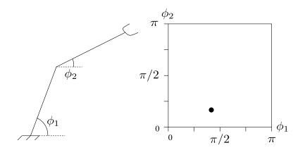
configuration space of a two-arm robot moving in the 2-dimensional plane
