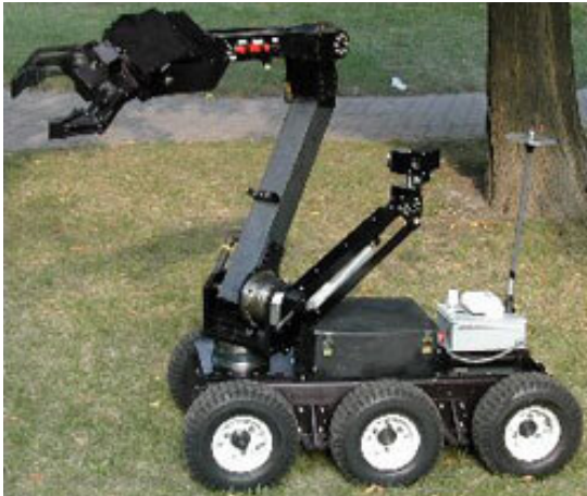
the MR-5 mobile robot (Engineering Services Inc.) used for demining, SWAT and surveillance (tele-operated)
