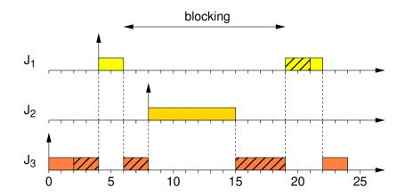
task J1 is blocked for the whole duration of a medium priority task that does not even require the blocking resource
