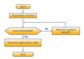
Adapted from https://en.wikipedia.org/wiki/Carrier-sense\_multiple\_access\_with\_collision\_avoidance
