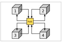
**Star ring** - Physical topology is star, the wiring inside hub makes the ring.
