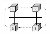
**Bus ring** (token bus) - Stations are connected to single cable called bus, but make logical ring.
