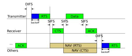
Network Allocation Vector (NAV) = Time set by other nodes after having received the duration of the transmission from the transmitter.
