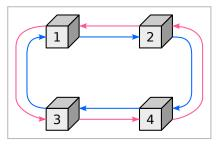
**Dual ring** - Uses second ring which operates in reverse direction.
