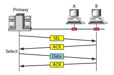
**Select** - The primary device wants to send data to secondary device, secondary device gets ready to receive.
