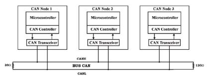
Architecture of the CAN bus according to the ISO 11898 standard. The standard allows up to 40 nodes to be connected to the same wire.
