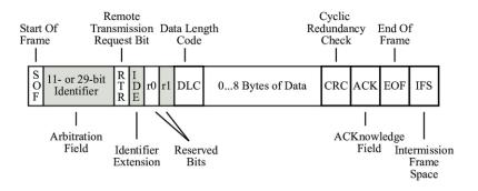
The identifier can use 11 bits (standard lenght) or 29 bits (extended length).
