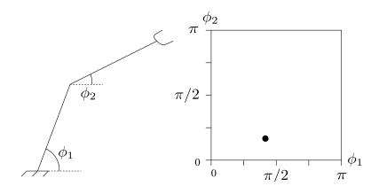
configuration space of a two-arm robot moving in the 2-dimensional plane
