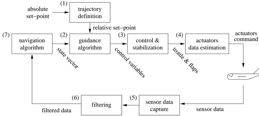
Fig. 3. Block diagram of the control application.
